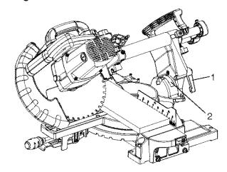
**NOTE:** The saw comes with a 33.9° crown molding stop.
